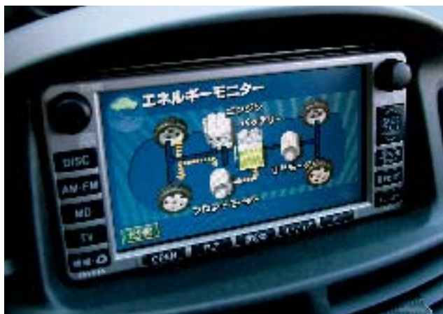
Voltage view: An in-dash display shows a hybrid's electricity flows.
